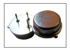
It is a true one-port SAW resonator in a low profile TO39 case. This product is designed for remote control and wireless security transmitters.
