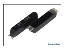
The tuning fork type quartz crystal provides ultimate in size, performance and economic tradeoffs. So, it is used as a clock source in communication equipment, measuring instruments, microprocessors and other time management applications.
